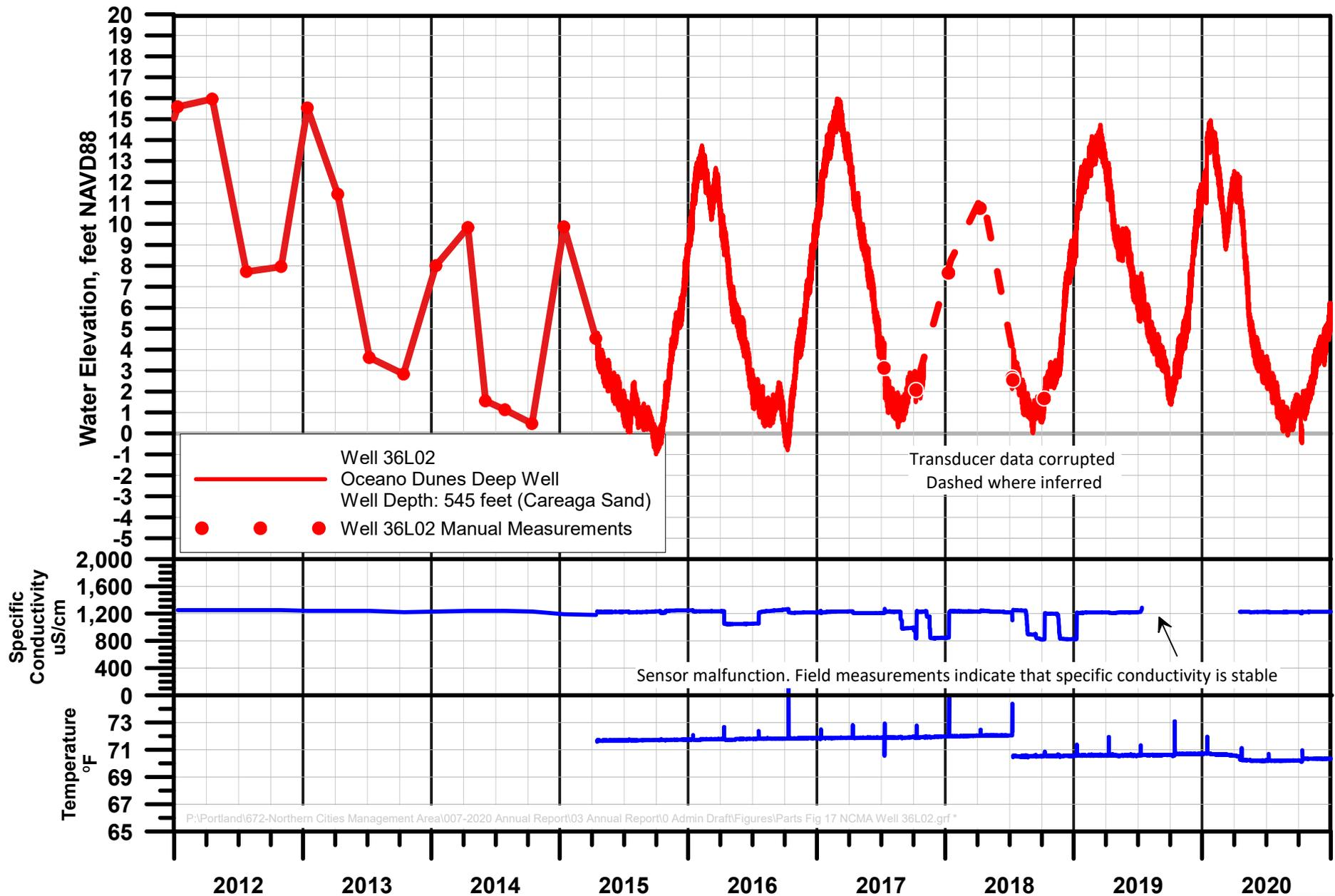
**FIGURE 17. WATER ELEVATION, CONDUCTIVITY, AND TEMPERATURE, WELL 36L02**
