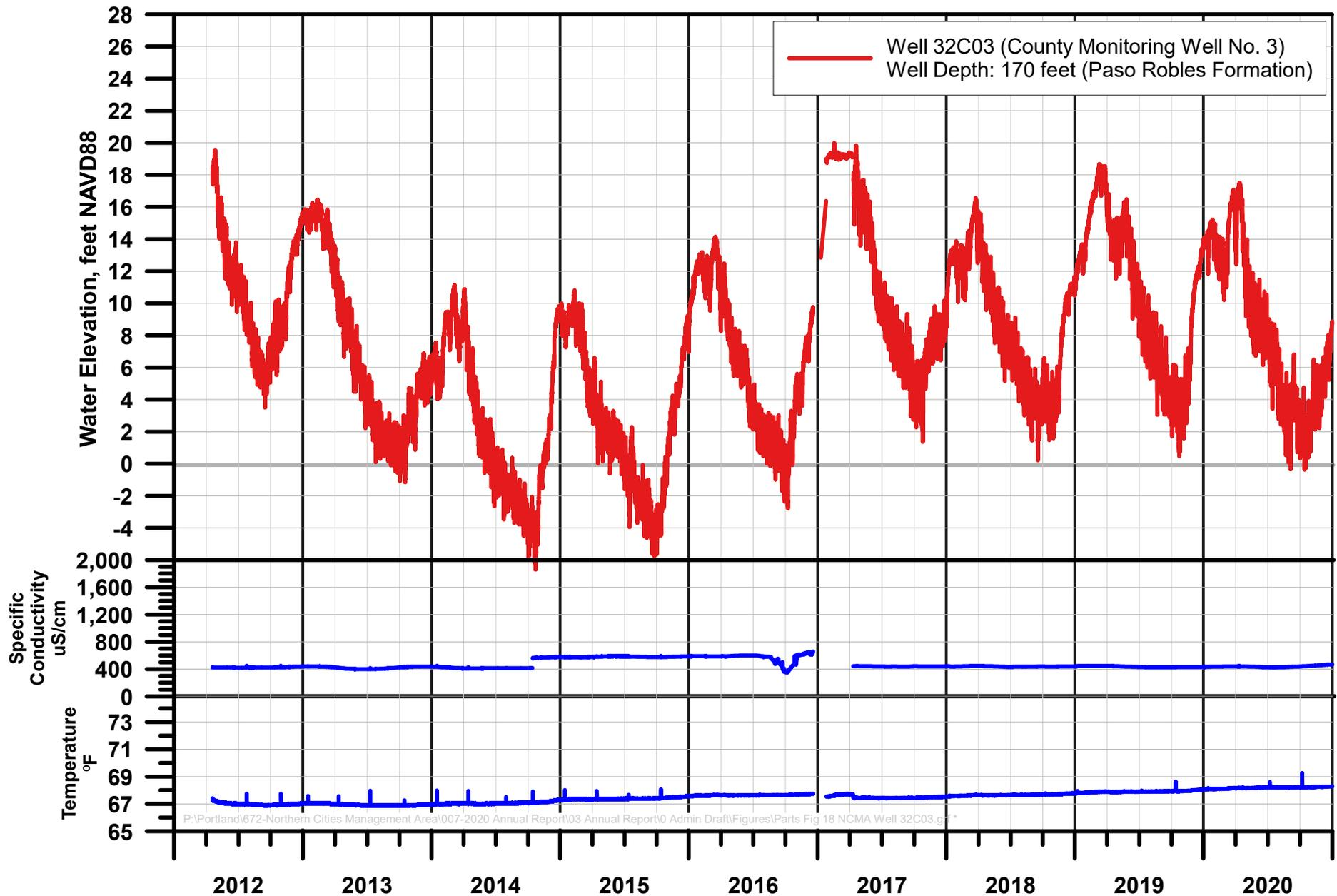
**FIGURE 18. WATER ELEVATION, CONDUCTIVITY, AND TEMPERATURE, WELL 32C03**
