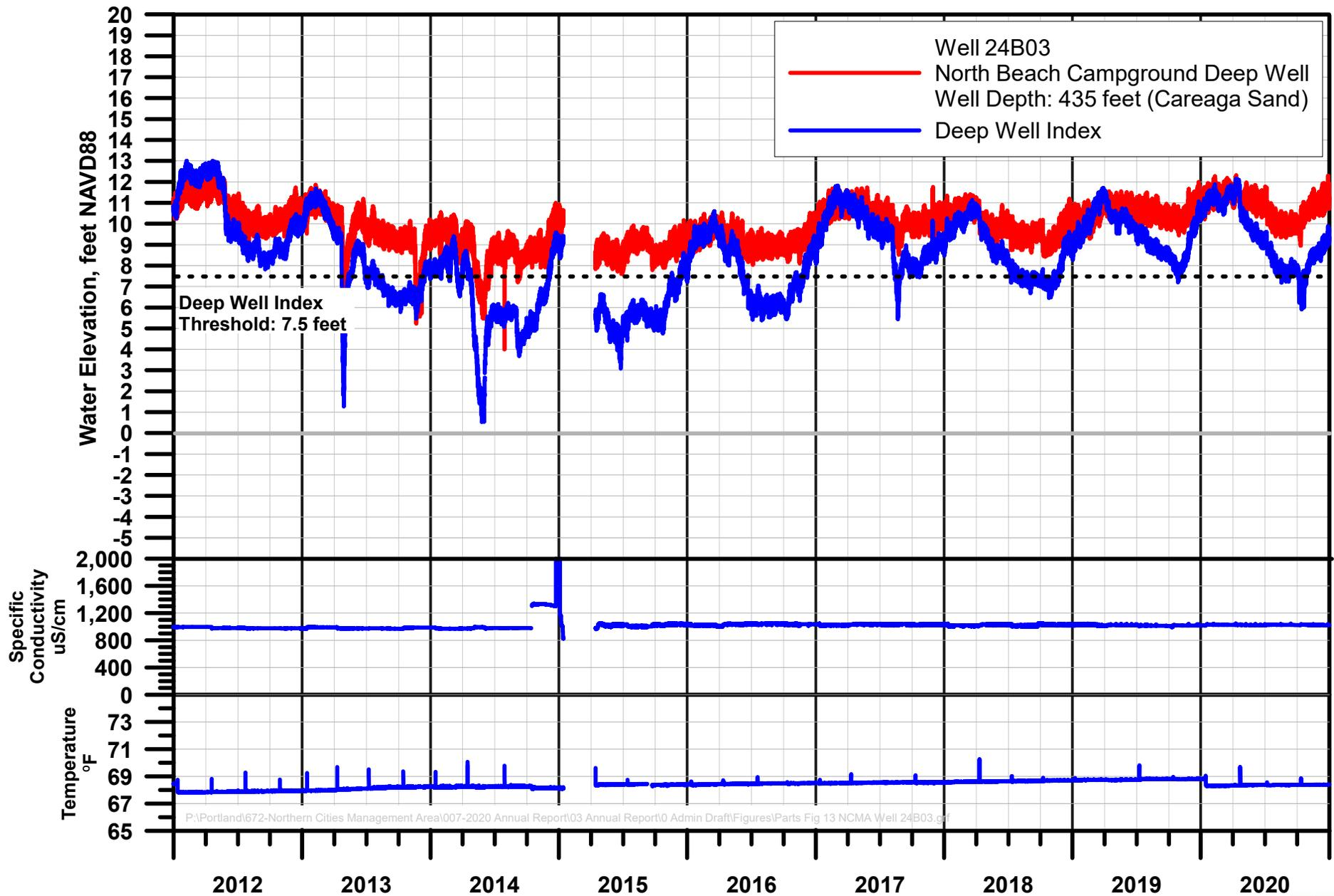
**FIGURE 13. WATER ELEVATION, CONDUCTIVITY, AND TEMPERATURE, WELL 24B03**
