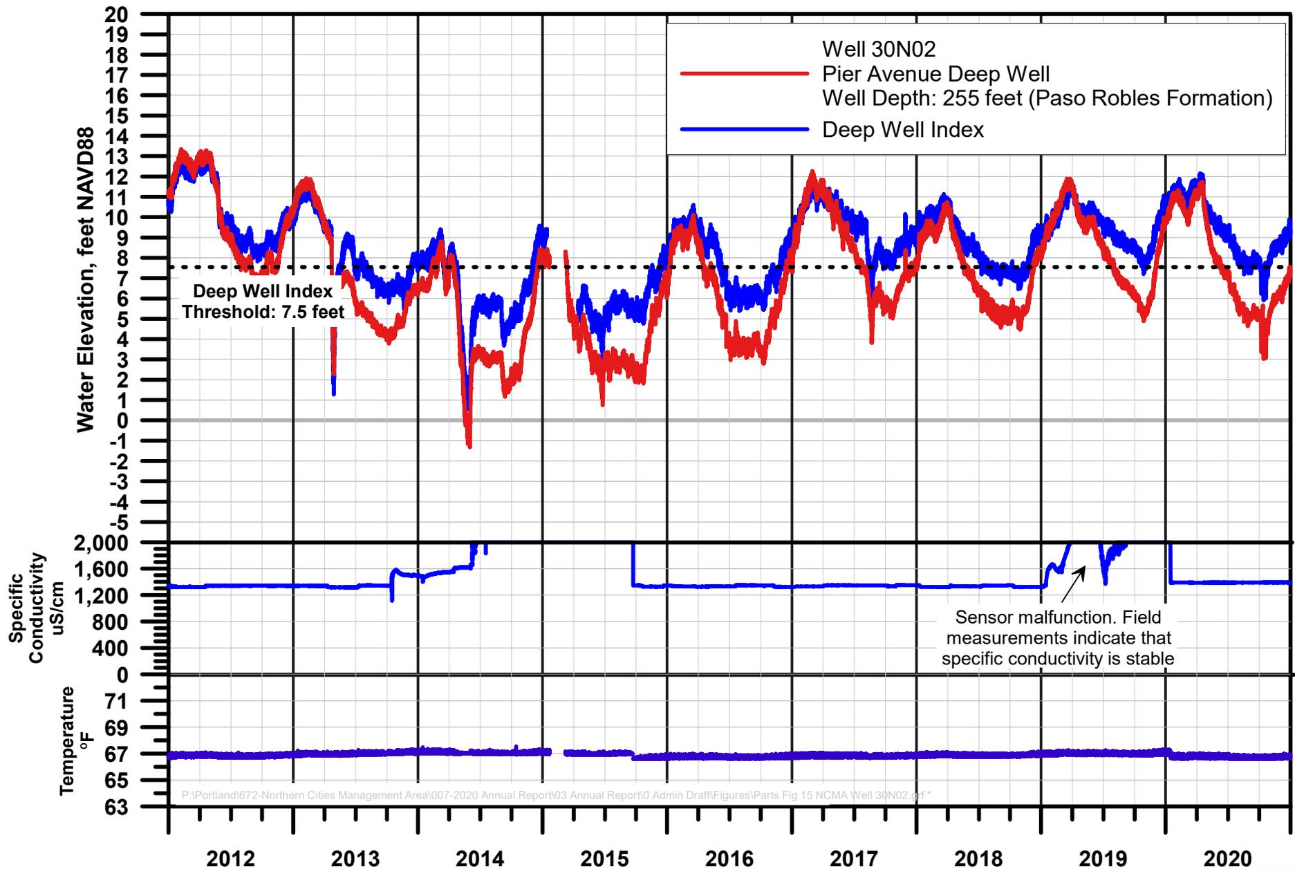
**FIGURE 15. WATER ELEVATION, CONDUCTIVITY, AND TEMPERATURE, WELL 30N02**
